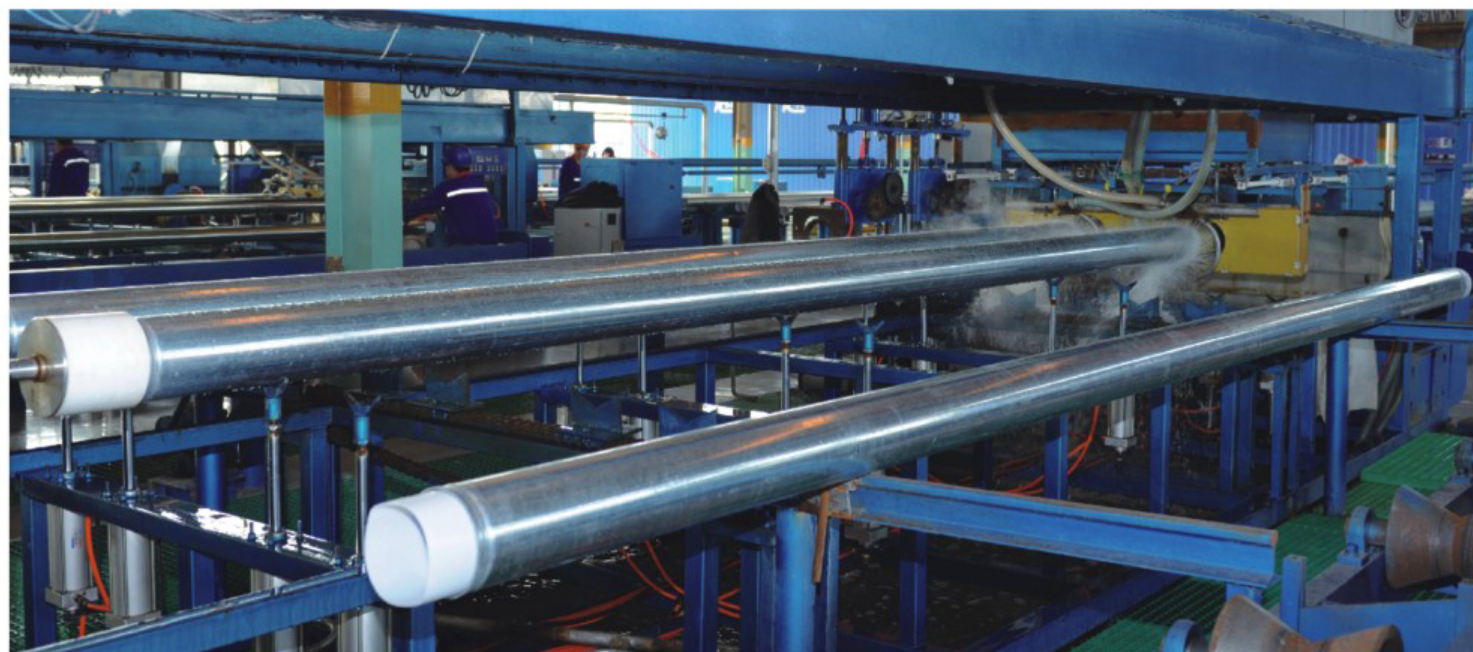
Steel Pipe of Lining Plastic Production Line
